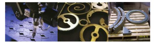
This machine is capable of cutting up to 150mm of mild steel & up to 120mm of various stainless steel with a mixture of High Pressure Water and Microblast Granite.
